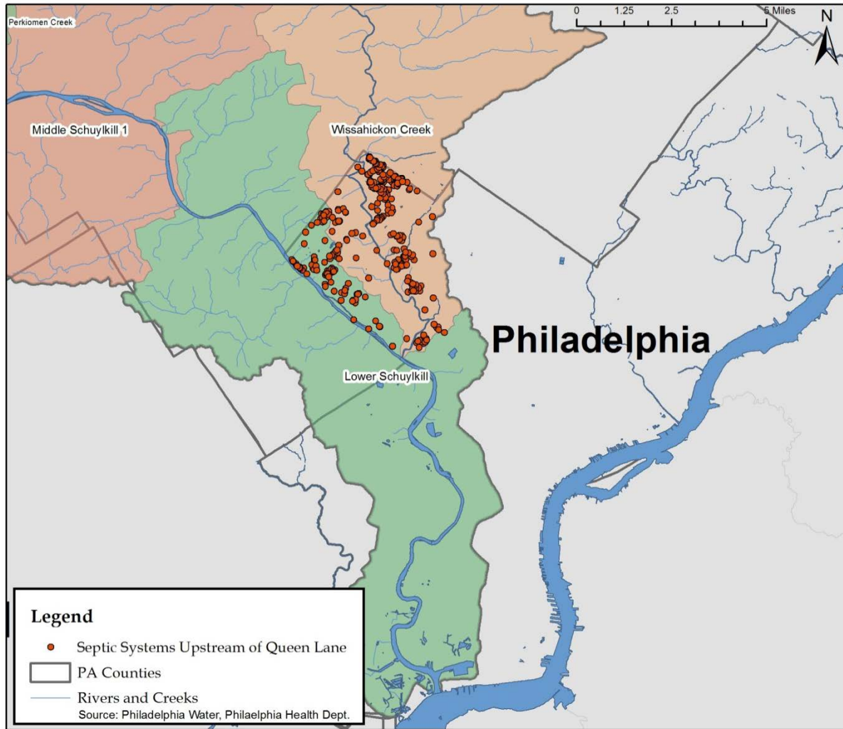
FIGURE 3-4: MAP OF SEPTIC SYSTEMS IN PHILADELPHIA COUNTY UPSTREAM OF QUEEN LANE WATER TREATMENT PLANT
